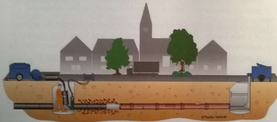
Figure 8.21 Installation of new water mains using trenchless techniques. The old pipe is broken by a device operated from an access hole. Excavation near to tree roots will be minimised.
